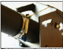
Tighten the clip as tight as you can without deforming the tube, the wire loop will press into the tube; this is OK.
